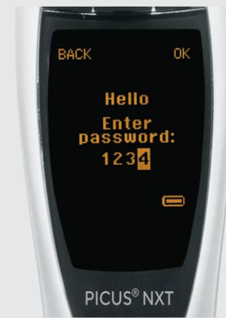
Fig 1. Picus® NxT password protection option on display
