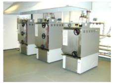
All of this makes buying, specifying, installing and running a laboratory autoclave more difficult than it used to be. Gone are the days when you could look through a catalogue to pick one out and once it was delivered, plug it in with a bucket behind to catch the drips, or a pipe running into the nearest drain or through the wall, set it to 15 minutes at 121°C and empty it out again once there was no pressure inside.
